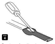
Then using a small screwdriver make an opening at the bulge.
