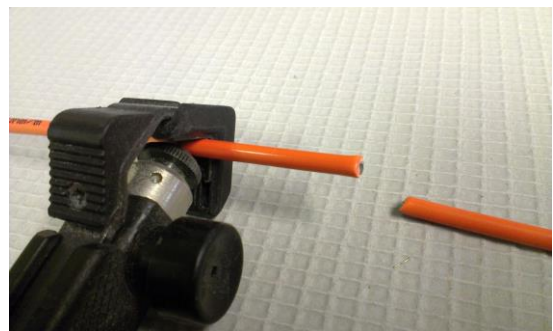
4) Strip 40mm of the outer sheath from each cable end.
