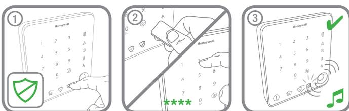
The Disarm button LED will always remain flashing throughout Test Mode. The Keypad will return back to Disarm Mode if no operation is made within 5 minutes of entering Test Mode. After performing a programming operation, press 0 to return back to the top level of Test Mode menu or
