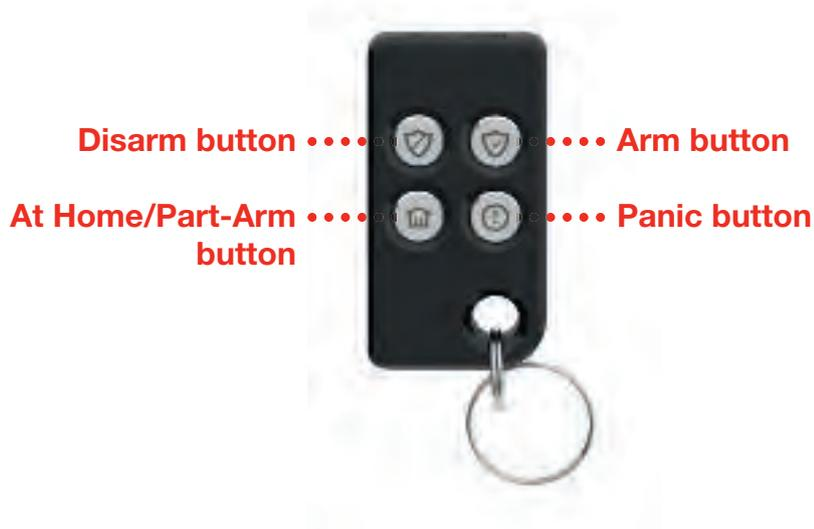
The Remote Control Fob also incorporates a Personal Attack (PA) button. Pressing and holding the Panic button for 3 seconds will immediately trigger an Alarm (unless the Keypad is in Test or Program Modes) even if the system is disarmed. The alarm can be cancelled using the Remote Control by pressing the 'DISARM' button.
