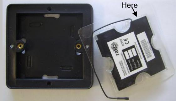
Unscrew and remove Front from Wall plate
