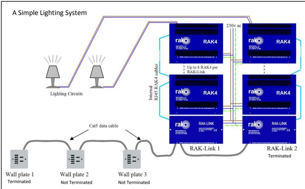
This picture shows a simple lighting installation using the Rako Wired system.
