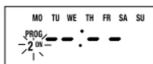
The TG77 now has the first programme locked into memory and is ready to receive additional programmes if required. When programming is complete press the TIME button to return to the operating mode. When programming additional programmes the choice of day or day group is always totally open.
